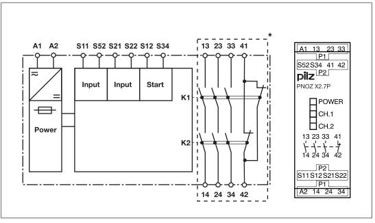
\*Insulation between the non-marked area and the relay contacts: Basic insulation (overvoltage category III), Protective separation (overvoltage category II)
